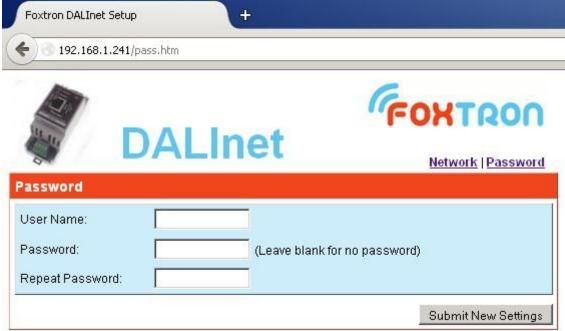
For password change fill the User name and twice new password. In the case that you do not want to use password leave the fields blank. By pressing "Submit New Settings" new password is saved.
