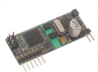
KNX232e is used for control and reading conditions on KNX bus
