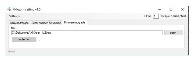
To overwrite the firmware in KNXpar choose file with new firmware (\*.hex) and with button "write fw" you start firmware overwrite.
