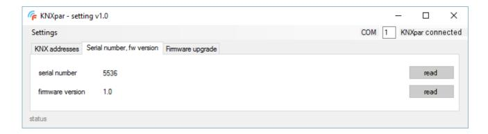
With "Read" buttons can be serial number and version read from KNXpar.
