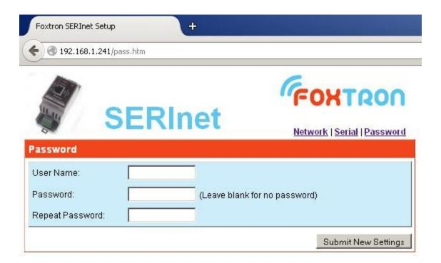
For change of password fill the User Name and twice new password. In the case that you do not want to use password leave the password fields blank. By pressing the button "Submit New Settings" you save new password.
